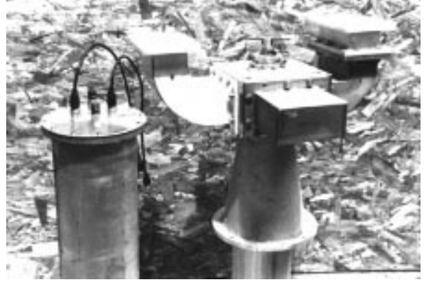
Fig. 12. Photograph comparing the size of an L -band disk turnstile with Dicke's full waveguide turnstile.
